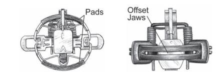
Double jaw traps use two metal frames instead of one. One set of jaws is smaller, and these are inside of the regular jaws.
