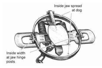
You can take these two measurements by setting the trap. Carefully measure the inside spread of the jaw frame at its widest point along the line from the dog to the opposite side. Then measure the width between the two jaws where they connect to the hinge posts. You may find slight differences in jaw spread measurements on the same make and model of traps.
