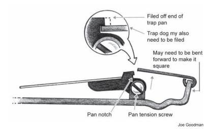
When the trap is set the trap pan should be level with the jaws. If the pan rests too high or too low you will need to bend the frame in or out below the "dog". Bend it out to raise the pan. Bend it in to lower the pan.
