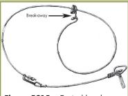
Figure EC15a. Typical breakaway
