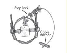
Figure EC14b. Powered cable device (set)
