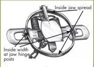
Figure EC3. Coil-spring trap
