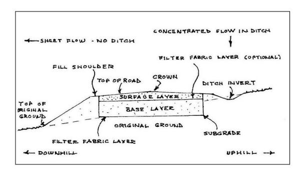
Figure 1 - Typical Road Cross-Section - Canaan, NH Highway Department
