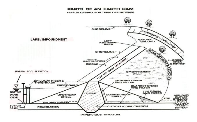
Fig. 10. Parts of an Earthen Dam (from Dam, Operation, Maintenance, and Inspection Manual – NCDENR Land Quality Section)
