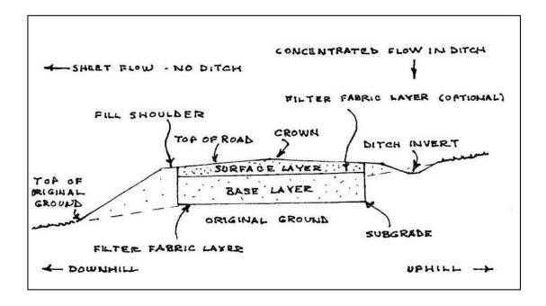
Fig. 9. Typical Road Cross-Section – Canaan, NH Highway Department
