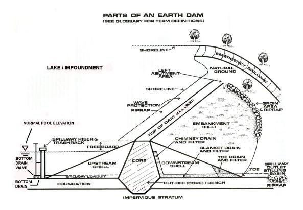
Figure 2 – Parts of an Earthen Dam (from Dam, Operation, Maintenance, and Inspection Manual – NCDENR Land Quality Section)
